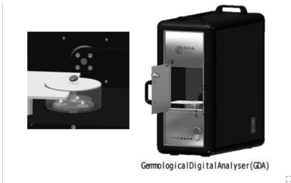
Fig. 1. Motorized rotation stage and mainframe of the GDA.
